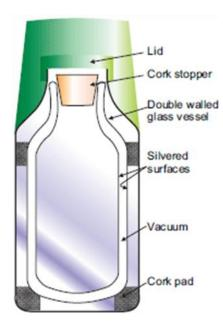
It has a thick stopper, double walls which are evacuated, and the vacuum bottle is silvered on the inside. Explain how this keeps drinks either hot or cold. What is the importance of each part of flask?
